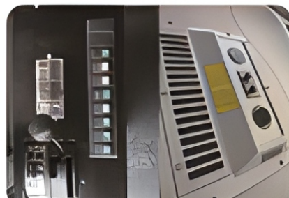
Simple control panel for easy key operation. The topmounted air-conditioning system enables the rapid adjustment of the cabin temperature.
