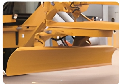
The action of the blade is controlled by full hydraulic pressure, and the blade can realize 360 ° rotation, telescopic expansion and contraction, and left and right 90 ° swing, which maximizes the equipment operating range and efficient construction.
